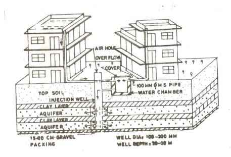
Drg-15: Gravity head recharge tube well
